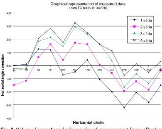
Fig. 6. Values of corrections for four series of measurement from calibration device in SIM
