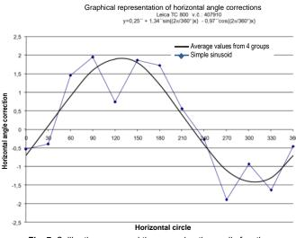
Fig. 7. Calibration curve and the approximating cyclic function
