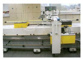
Fig. 1. Horizontal comparator
