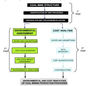
Fig. 2. The methodology framework of an algorithm for the development of the environmental and cost assessment of unit processes in a coal mine, proposed by the authors (source: own analysis)
