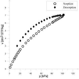
Fig. 3. Low pressure isotherm sorption/desorption of  $CO_2$  at 298 K
