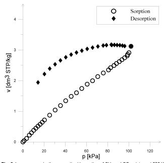
Fig. 5. Low pressure isotherm sorption/desorption of  $CH_4$  and  $CO_2$  mixture at 298 K
