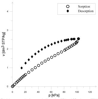
Fig. 6. Low pressure isotherm sorption/desorption of CH4 and CO2 mixture at 303 K
