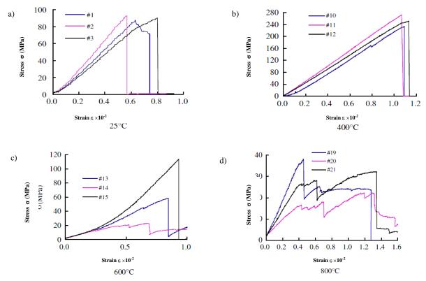
Figure 4. Stress-strain characteristics of mudstones: a - 25°C, b - 400°C, c - 600°C, d - 800°C (Zhang et al. 2013)
