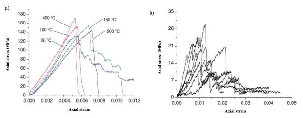
Figure 3. Stress-strain curves of sandstone samples: a - for temperatures in the range of 20-400°C, b - the temperature of 1200°C
