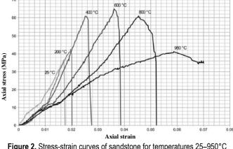
Figure 2. Stress-strain curves of sandstone for temperatures 25–950°C (Ranjith et al. 2012)
